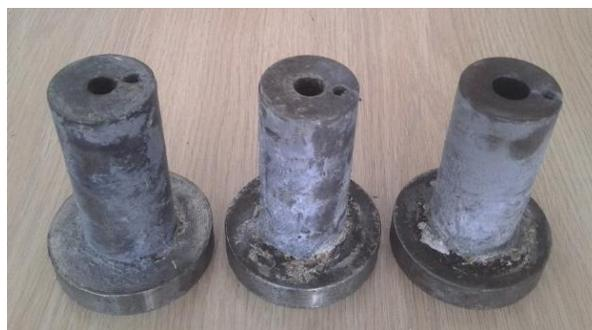
Fig 2: Compression molds with die hole diameter at 10mm, 12mm and 14mm
