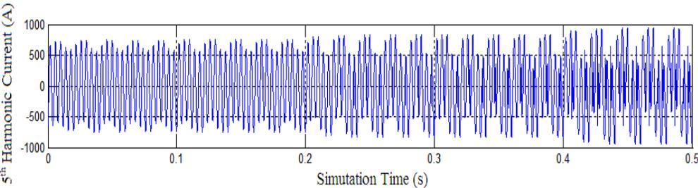
**Fig 3: 5th harmonic waveform of load current**
