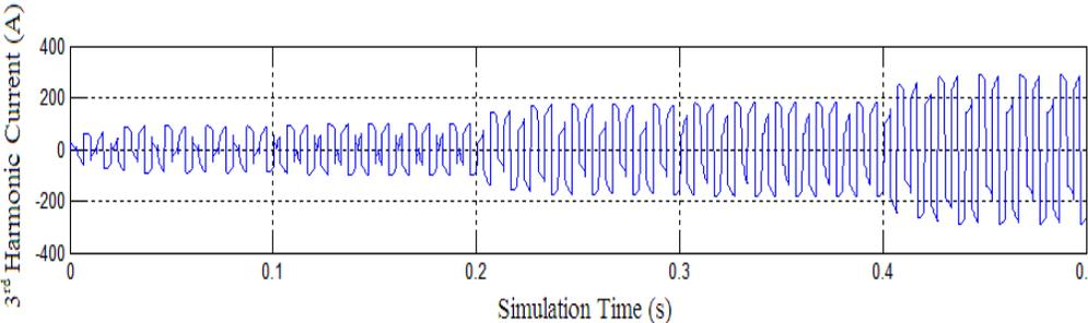
**Fig 2: 3rd harmonic waveform of load current**
