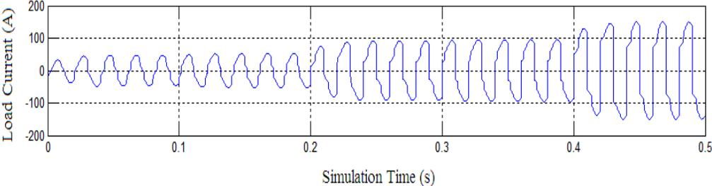
**Fig 1: Load current waveform of electrified railway**
