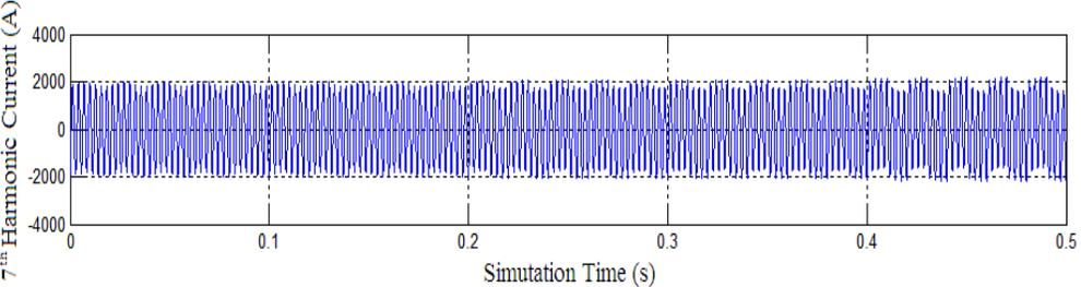
**Fig 4: 7th harmonic waveform of load current**
