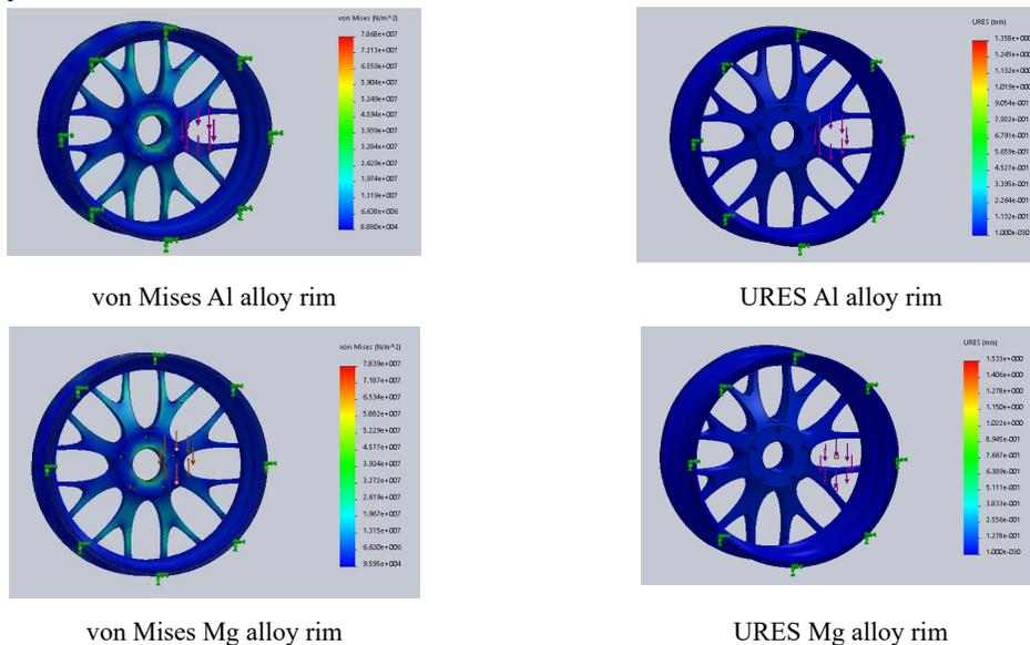
Fig 9: Von Mises stress and URES
