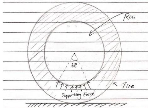
Fig 3: Illustrative figure of supporting force at the rim
