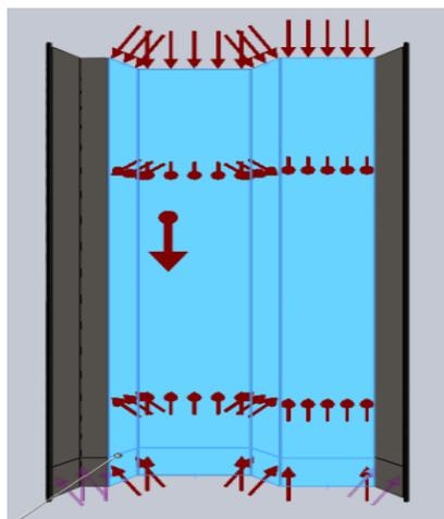
Fig 2: Tire pressure applied at retaining hump
