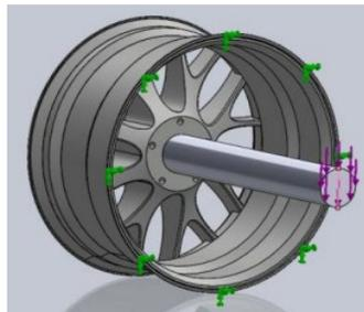
Fig 8: Basic set up of bending test
