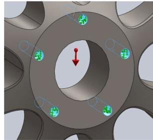
Fig 5: Bolt holes where the fixtures applied
