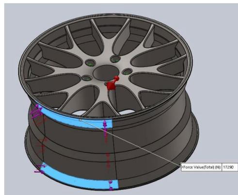
Fig 4: Applying loads at the split bead seats
