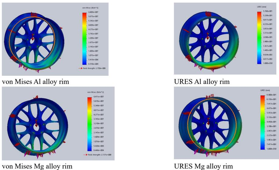
Fig 7: Von Mises stress and URES
